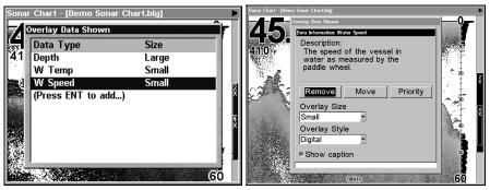
Overlay Data Shown, with water speed selected (left). Press ENT to access REMOVE option (right). Press ENT again to remove item and return to the Overlay Data Shown screen.
